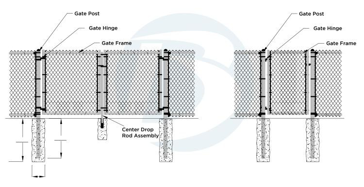
Notes: 1. If gate frame is not welded, a diagonal truss can be added.
